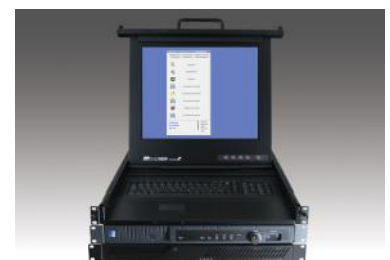
Crypto Management System rack-mountable server and security vault
